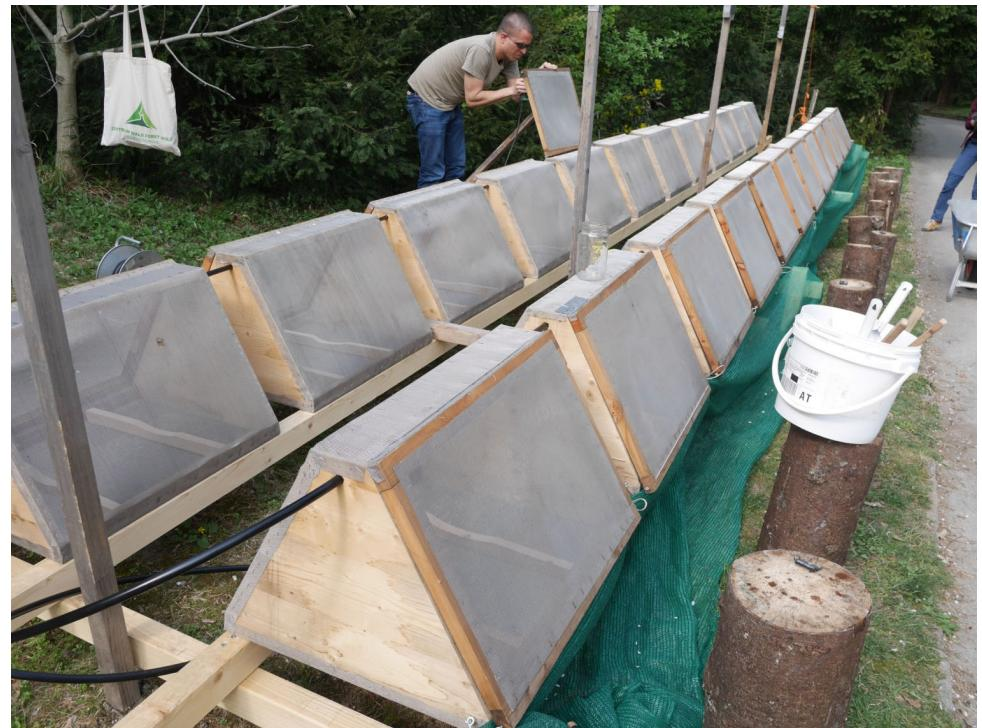
Experiment at BFW: Effect of irrigation on the emergence of *Ips typographus*
